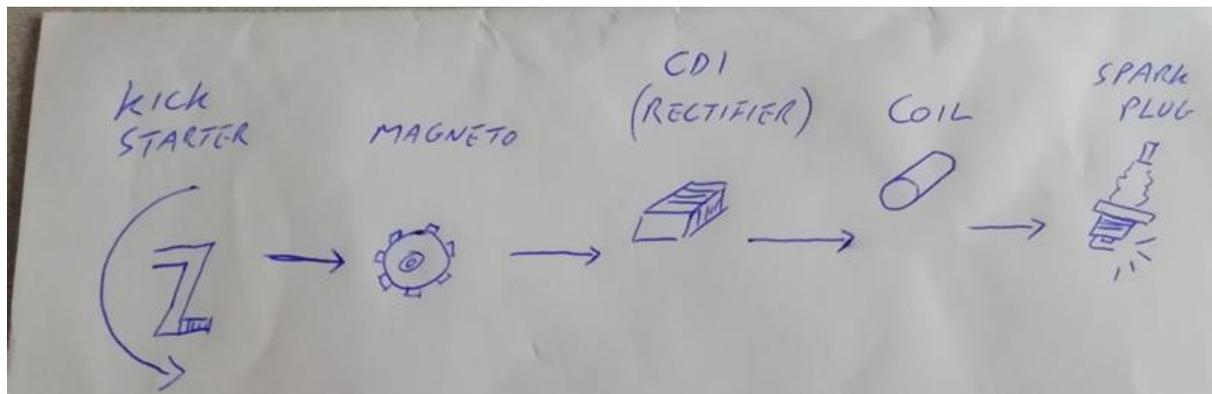
As the bike has no starter motor, it has to be started by kicking the kick start. This turns the magneto, which generates an AC current which then goes to the rectifier (or CDI) unit. This converts the power to DC, it also sends some electricity to the battery to keep it charged and generates the pulse for the spark plug. Electricity is then passed to the coil which converts or 'steps up' the charge to a higher charge and then sends pulses to the spark plug in the correct order.
